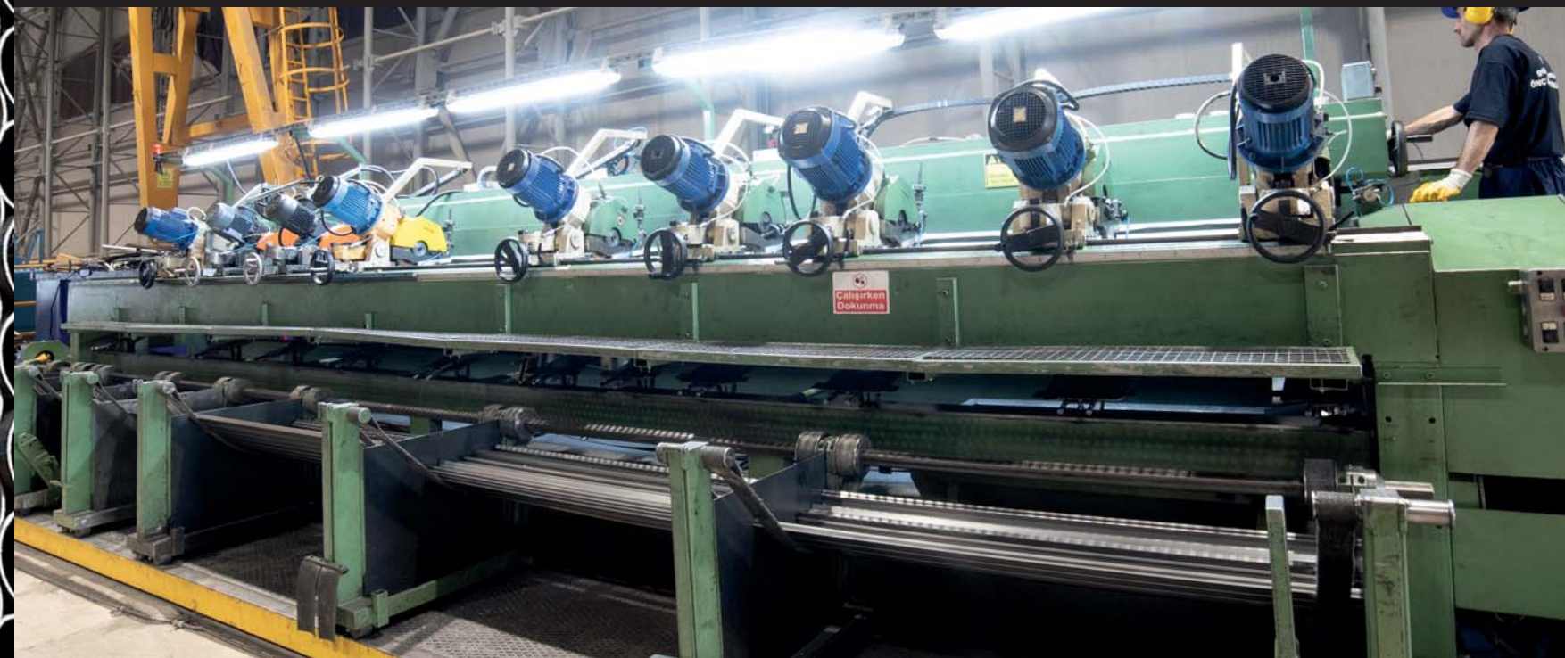
Multi-head tubes & profiles cutting machine Diameter: 13 mm - 51 mm Length: 475 mm - 7800 mm
